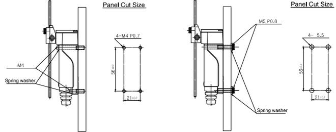
※ Hole depth must be 15mm(minimum).
