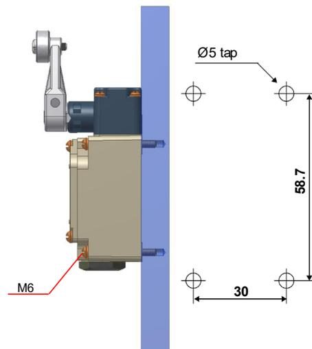
To install the Switch, make a mounting panel, as shown in the diagram
