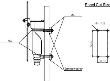
※ Maximum panel thickness must be less than 5mm.
